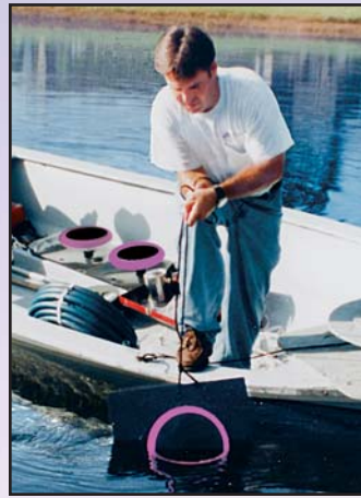
Technician placing Vertex AirStation™ into Heron Cay's lake.
