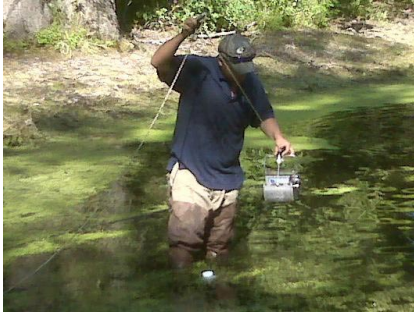
Figure 3. Preparing to use Eckman dredge
