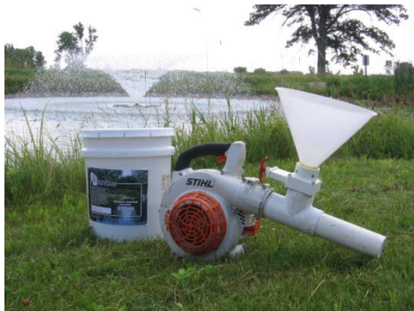
Figure 5. Picture of blower with hopper attachment used for bacteria application
